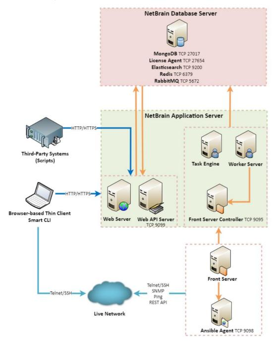
**Note:** The port numbers listed in the above architecture diagram are defaults only. The actual port numbers used during installation might be different.
