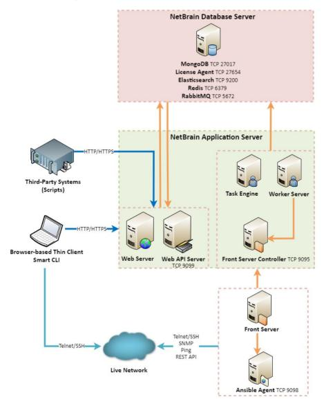
Note: The port numbers listed in the above architecture diagram are defaults only. The actual port numbers used during installation might be different.
