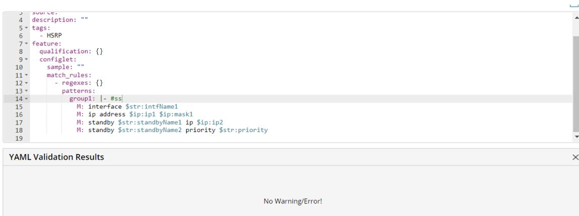
The screenshot shows a code editor with a YAML configuration snippet. The configuration includes a `match_rules` section with a `patterns` group containing four match rules. Below the code editor, a `YAML Validation Results` window is open, displaying the message "No Warning/Error!".
